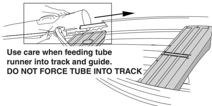
Use care when feeding tube runner into track and guide. **DO NOT FORCE TUBE INTO TRACK**
