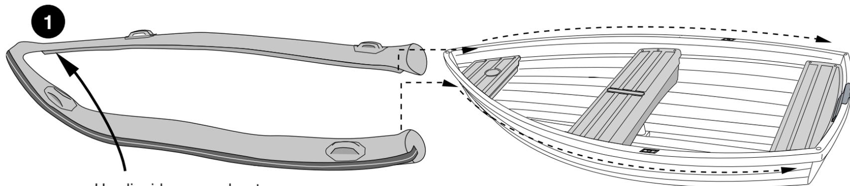
Use liquid soap and water on the track runner on the tube to help slide the tube on with greater ease.
